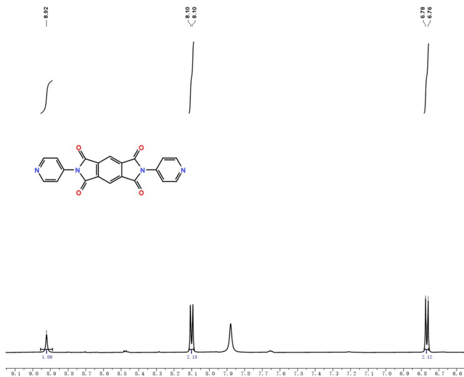
Figure S1. ^1\text{H} NMR spectra of N' -bis(4-aminopyridine)phenylenediimide in \text{CDCl}_3 at room temperature.
