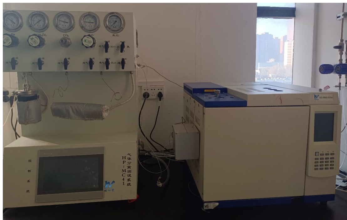
Fig. S14 The homemade HPMC41 gas separation test system.
