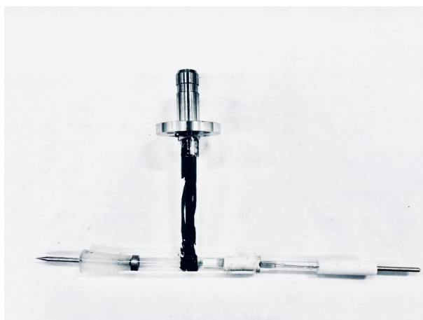
Figure S17. The experimental device of tee quartz tube for neutron diffraction.
