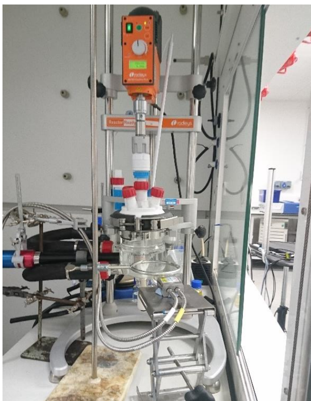
Figure S16 Photograph of setup for Experiment 4, showing 250 mL STR with non-invasive Raman monitoring from the Kaiser PhAT probe and Tornado Hudson.
