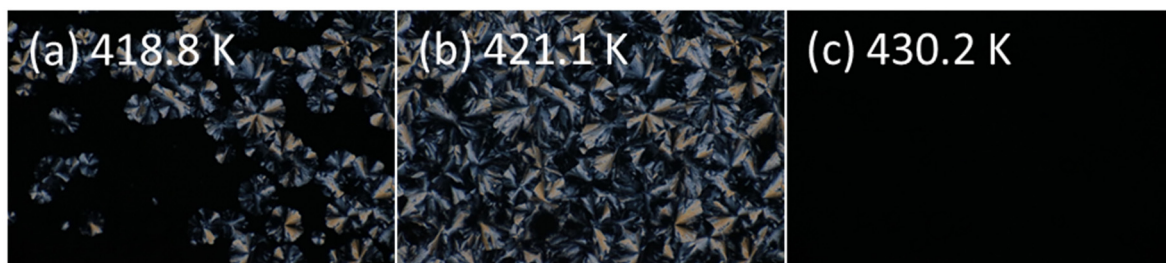
Fig. S4. Microphotographs for the mixture of Bis-B10Si2 and 10 mol% PDMS under crossed polarizers at (a) 418.8 K (around the Cub to Col h phase transition), (b) 421.1 K (Col h ), (d) 430.2 K (Iso) on heating.
