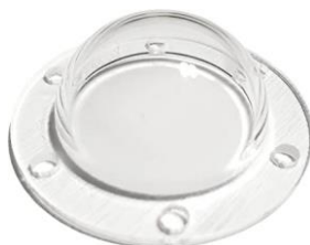
Figure S1. Template for making spectroscopic mini-chamber: transparent hollow hemisphere.
