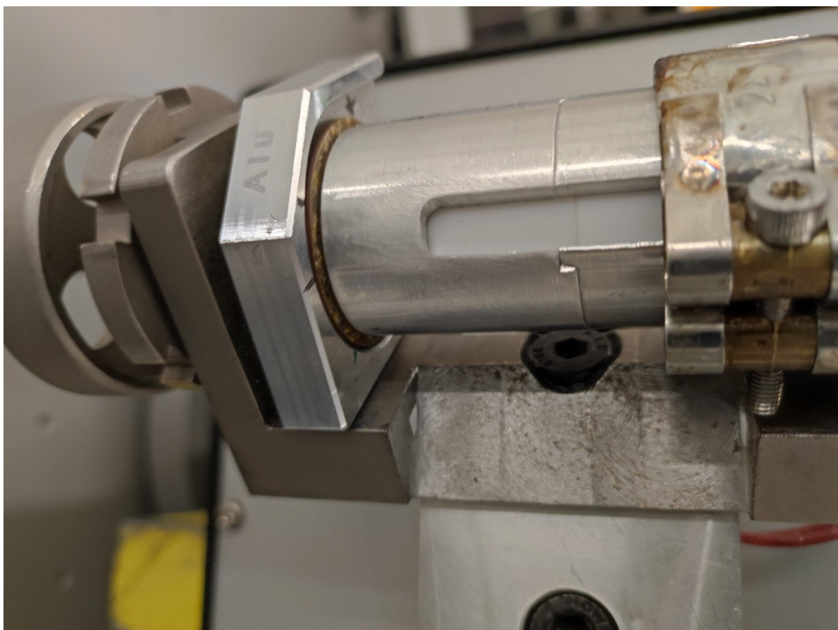
Fig. S7. Front view of our thermo-mechanochemical reaction setup at DESY synchrotron. Jar size is 8 cm in length.
