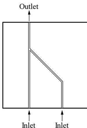
Figure S1 Schematic diagram of the channels of the droplet generator.
