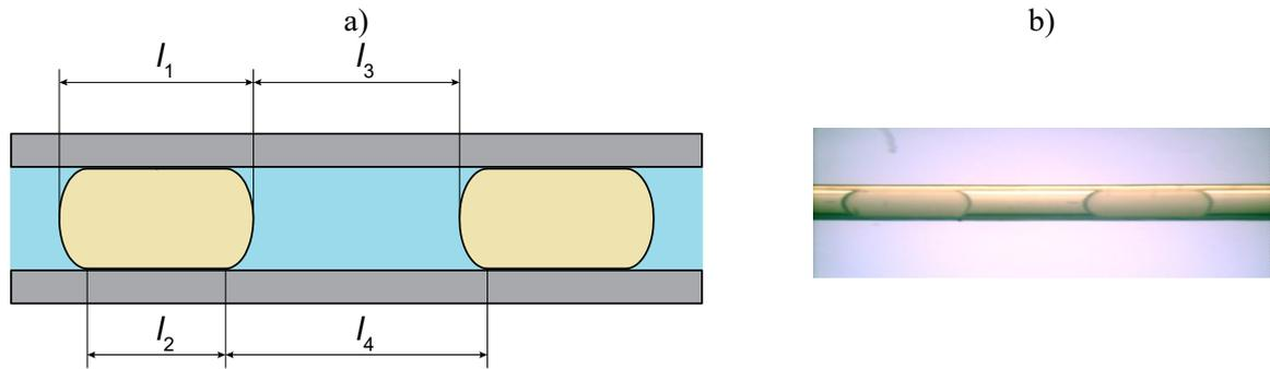
Figure S2 a) Measured droplet parameters of the aqueous ( $l_1, l_2$ ) and organic ( $l_3, l_4$ ) phases, b) microscope image of obtained droplets.
