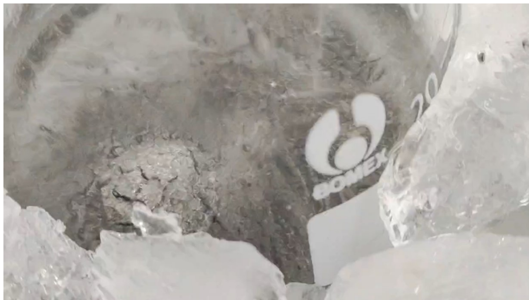
Fig. S2 (video). The reaction process of Al/Bi/CNT on the ice.
