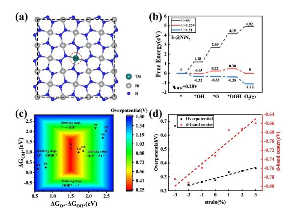
Single Ir atom embedded into  $NiN_2$  monolayer exhibit high OER catalytic activity with 0.28 eV overpotential. The OER catalytic activity of Ir atom embedded into  $NiN_2$  monolayer can further enhanced by strain.
