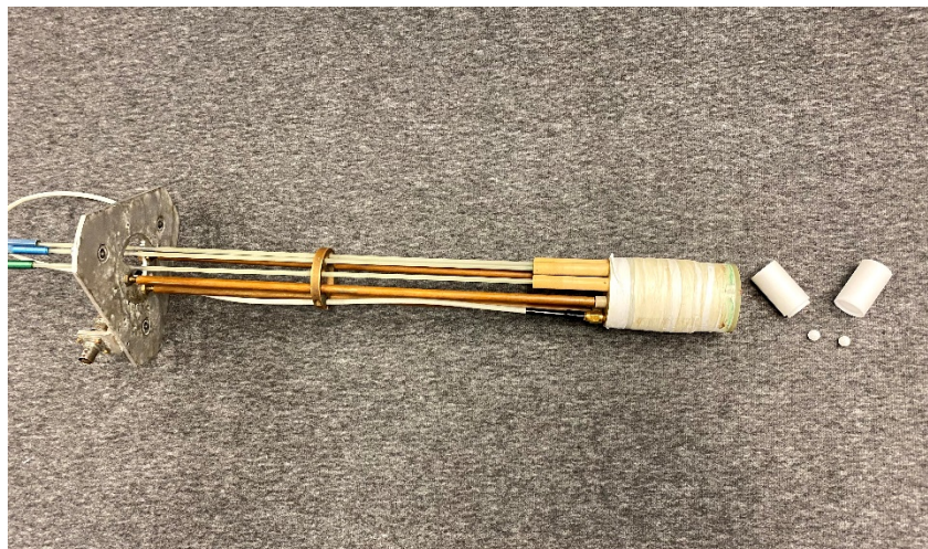
Figure S1. Doty DS1-874 ^1\text{H} RF probe, small 7.5 mL Teflon jar, and two small 7 mm zirconia balls.
