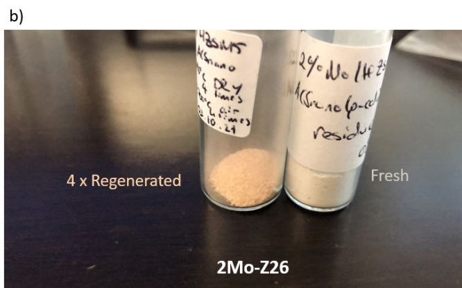
Figure S17. The color change of samples before and after reaction-regeneration cycles: a) 2W-Z26 and b) 2Mo-Z26
