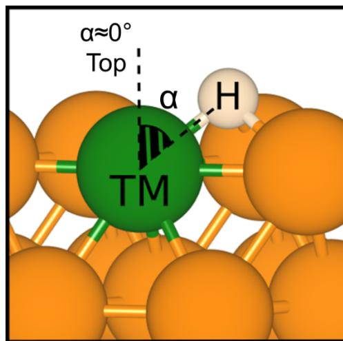
**Figure S1:** Definition of the angle  $\alpha$  between the H atom and the normal to the TM atom on the surface.
