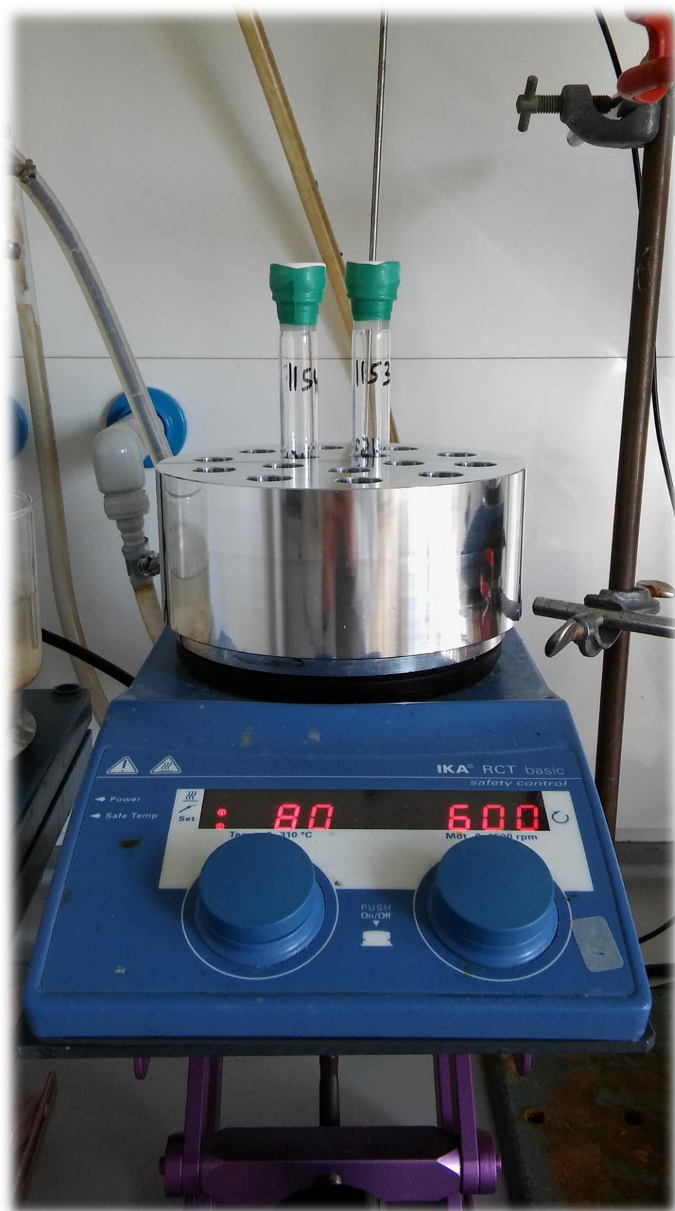
Figure S4. Stirring of the reaction mixture at appropriate temperature.
