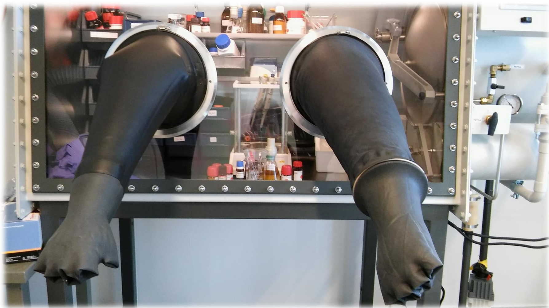
Figure S2. Charging of reaction vials with solid reactants and catalyst in the glovebox.
