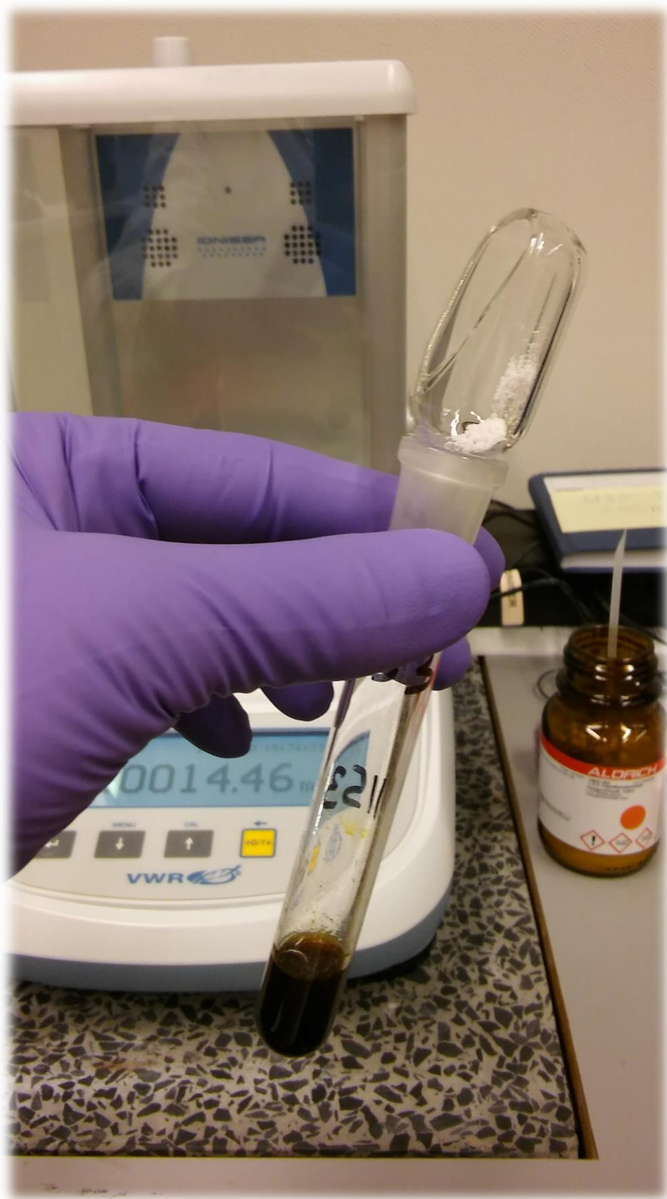
Figure S5. Addition of an internal standard to the reaction mixture at room temperature.
