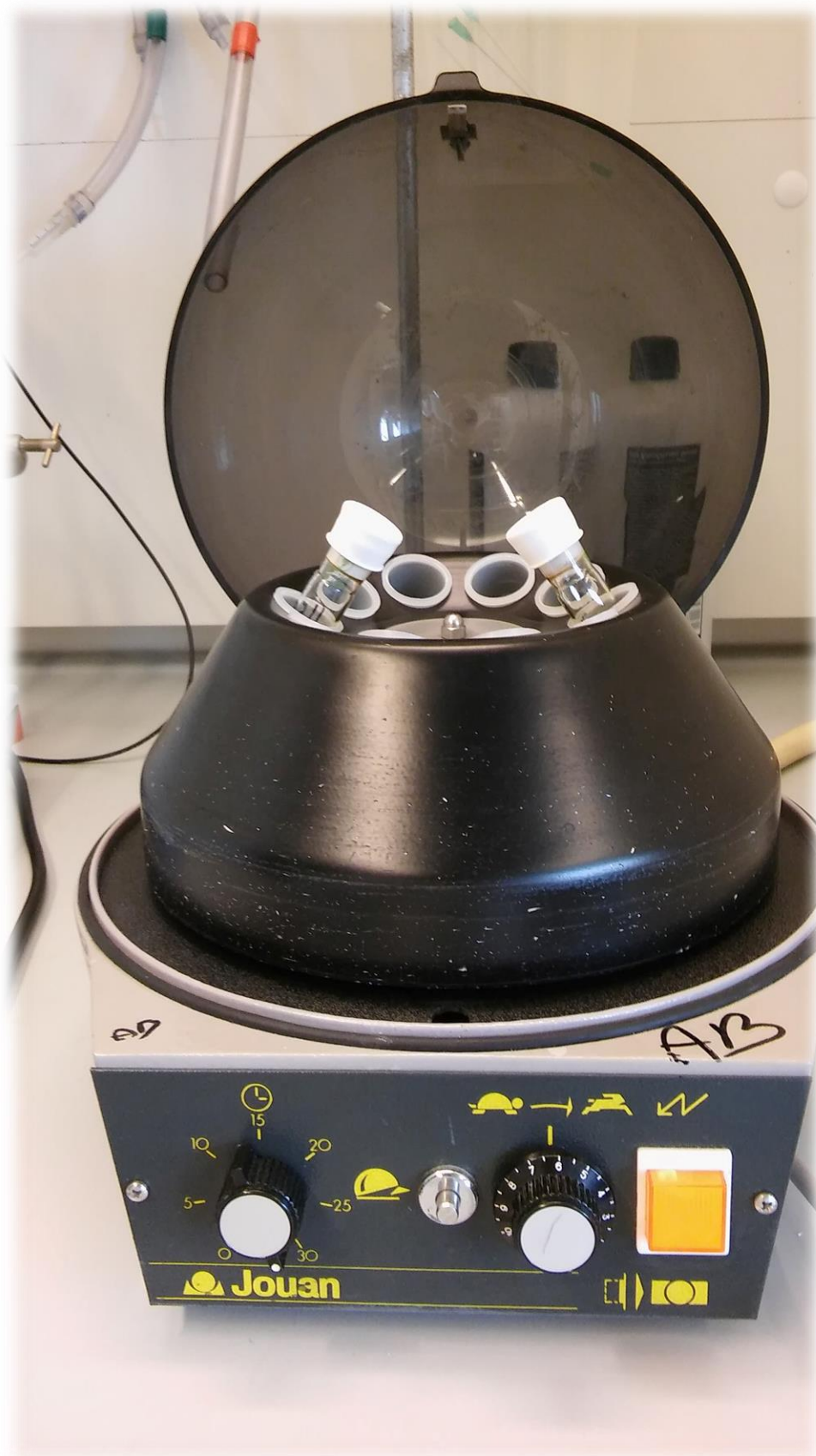
Figure S8. Centrifugation to precipitate the inorganic matter.
