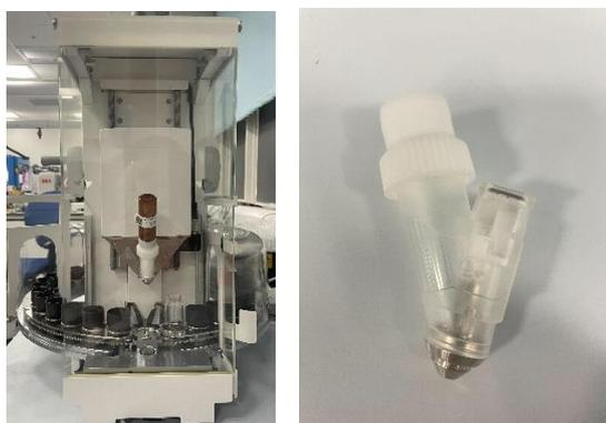
**Figure S1.** Quantos XPE206 dosing system (left) and QH008-BNMW dosing head (right).
