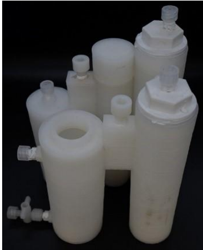
Figure 14. An example of a monolithic reactor fitted with non-printed elements
