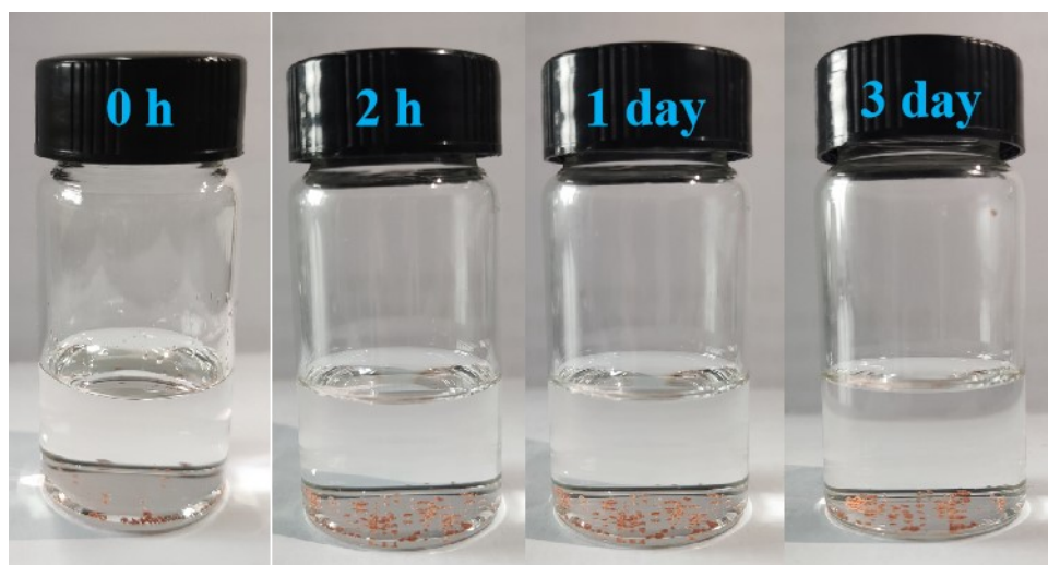
Figure S4. Photographs of Co-DTBPT soaked in the electrolyte for different time durations.
