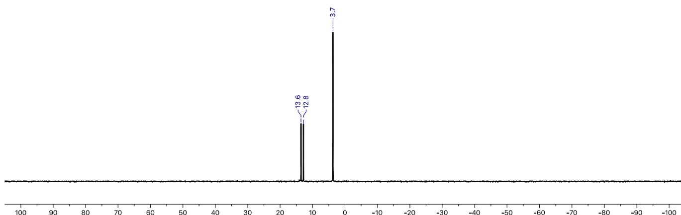
**Figure S11.**  $^{31}\text{P}\{^1\text{H}\}$  NMR spectrum of **1-OH<sub>2</sub>** with internal  $\text{O}=\text{P}(\text{OMe})_3$  standard ( $\text{CD}_2\text{Cl}_2$ , 162 MHz).
