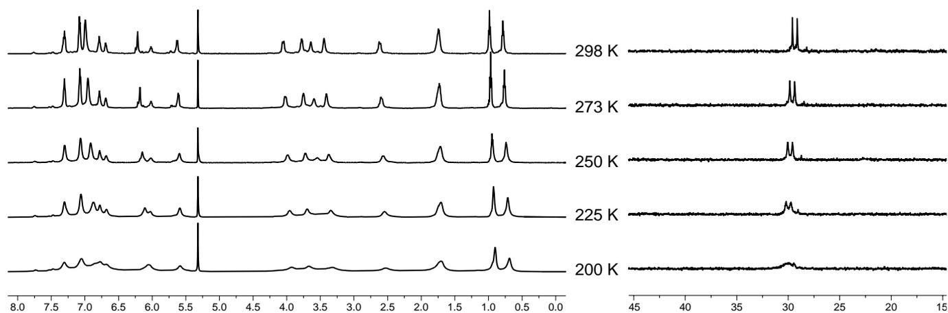
**Figure S4.** Variable temperature  $^1\text{H}$  and  $^{31}\text{P}\{^1\text{H}\}$  NMR spectra of **2** ( $\text{CD}_2\text{Cl}_2$ , 600/243 MHz).
