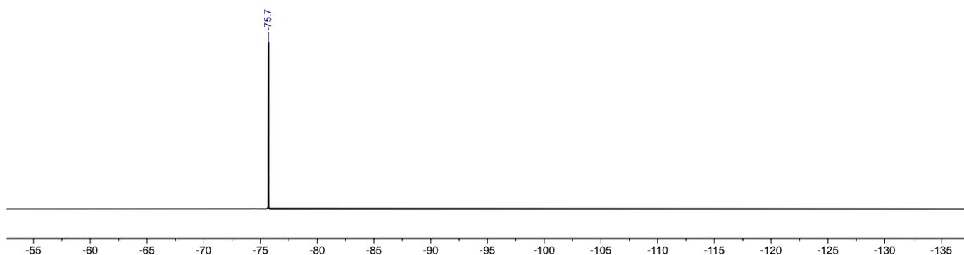
**Figure S10.**  $^{19}\text{F}\{^1\text{H}\}$  NMR spectrum of **1-ClAg** ( $\text{CD}_2\text{Cl}_2$ , 377 MHz).
