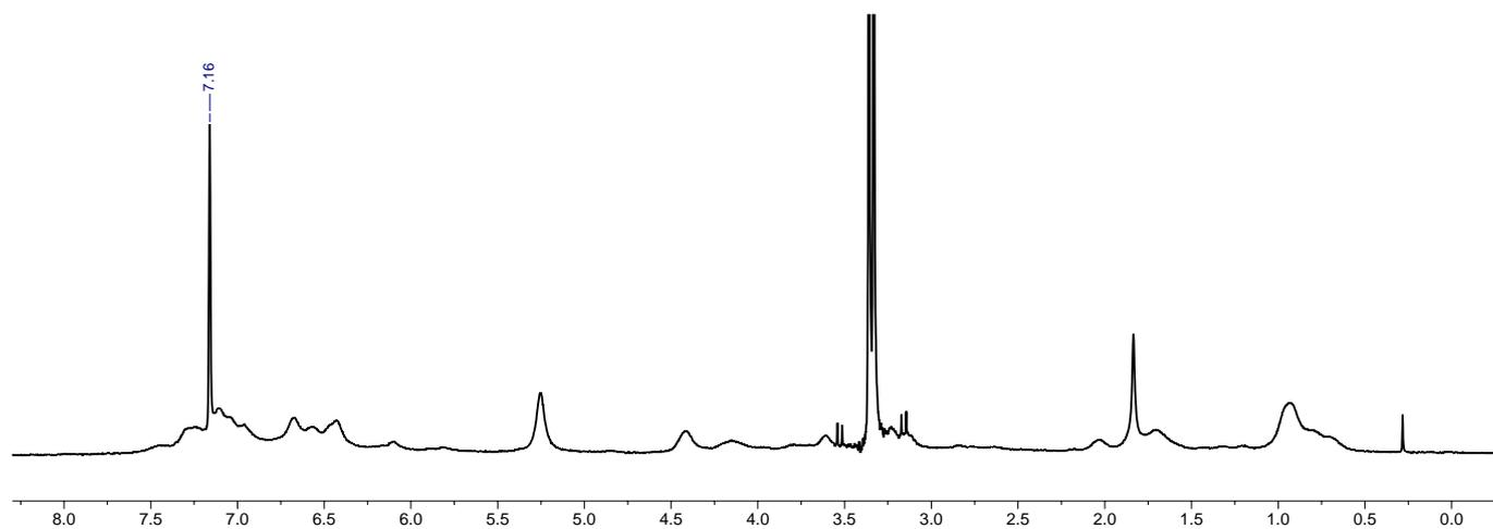
**Figure S5.**  $^1\text{H}$  NMR spectrum collected during the reaction between **2** and  $\text{Ag}[\text{Al}(\text{OR}^{\text{F}})_4]$  with internal  $\text{O}=\text{P}(\text{OMe})_3$  standard ( $\text{CD}_2\text{Cl}_2$ , 400 MHz).
