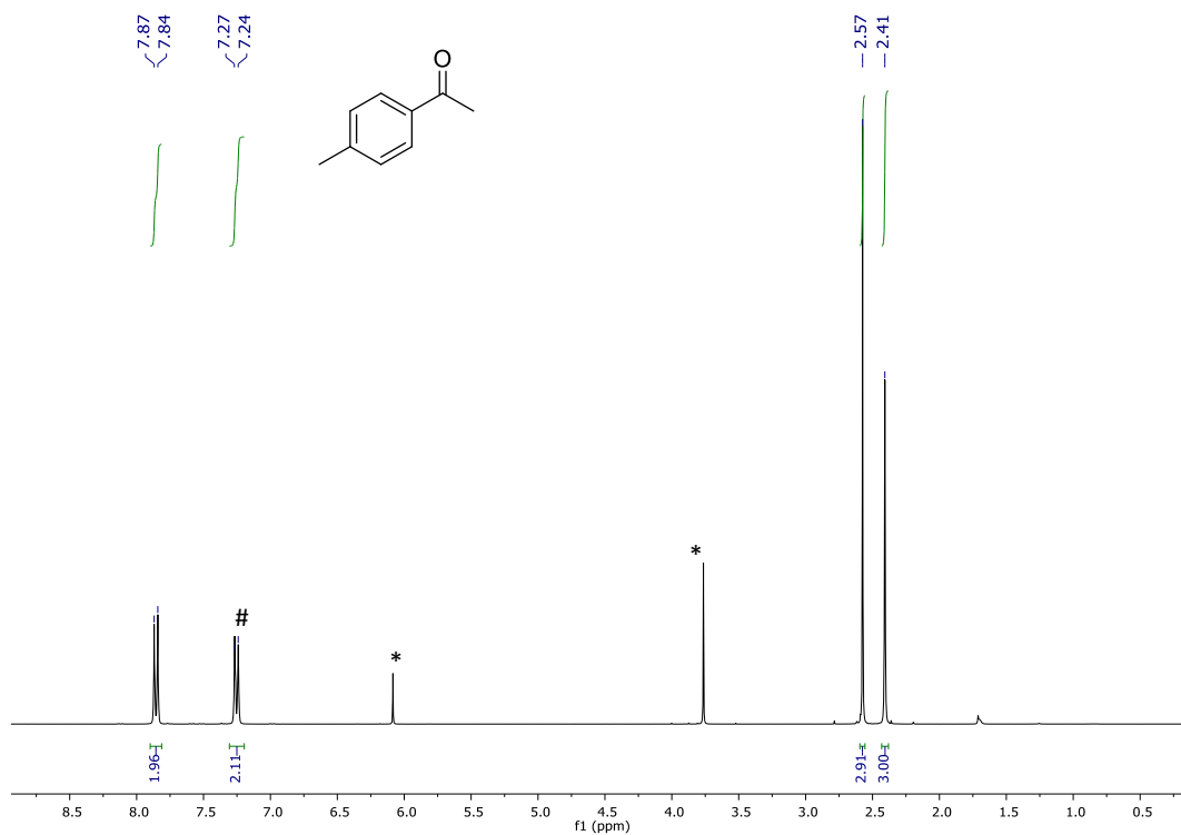
Figure S15. ^1\text{H} NMR spectrum ( \text{CDCl}_3 , 300MHz) of 4'-methylacetophenone (81% yield, from oxidation of 5b ; # \text{CHCl}_3 overlapping with a signal of the product, * internal standard: 1,3,5-trimethoxybenzene).
