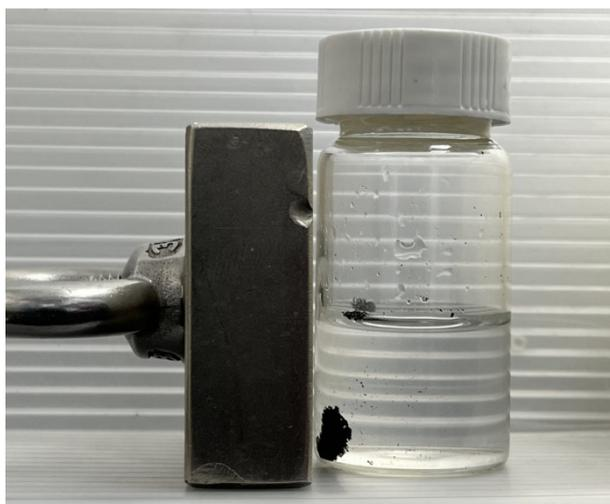
Figure S1. Recovery of adsorbents by the external magnetic field.
