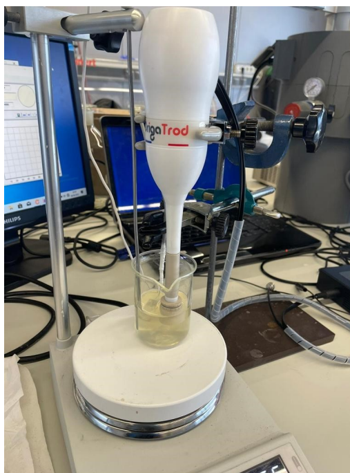
Figure S 1. Real anodization device, including rotating disk electrode and hot plate stirrer.
