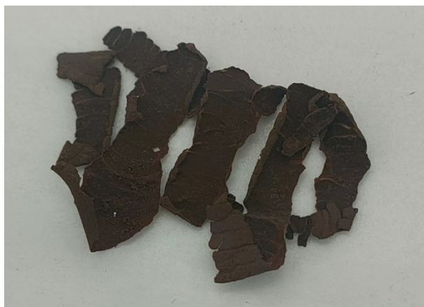
Fig. S7. Digital image of fractured, incomplete PIC with extremely poor flexibility.
