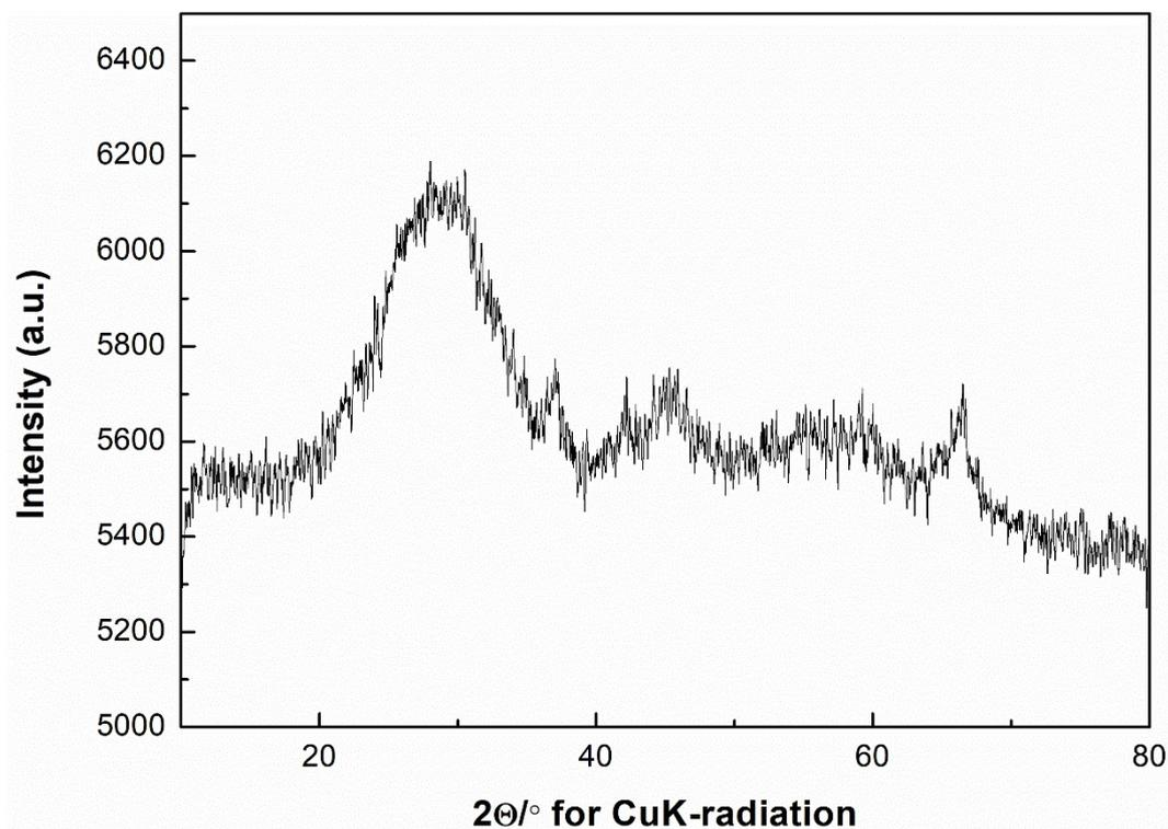
**Figure S4.** X-ray diffractogram of re-used VO<sub>2</sub> nano-urchin catalyst.
