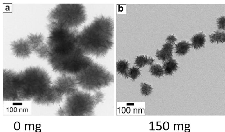
**Figure S1.** Transmission electron microscopy images showing the influence of amount of surfactant F-127 on the morphology of VO<sub>x</sub> nanourchins synthesized without F-127, (a) and 150 mg of F-127(b)
