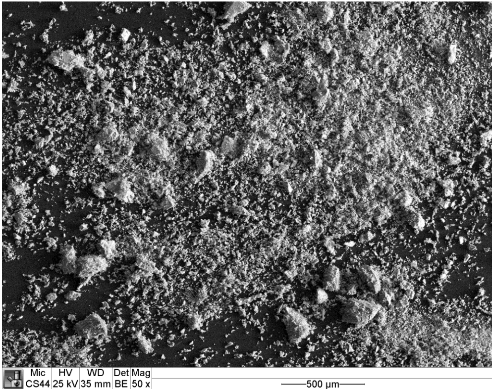
Figure S11: Scanning electron microscopic image of \text{Li}_{3.74}\text{Mg}_{0.13}\text{P}_2\text{S}_6 . The back scattered image detector is used to produce the image and the image is 50 times magnified.
