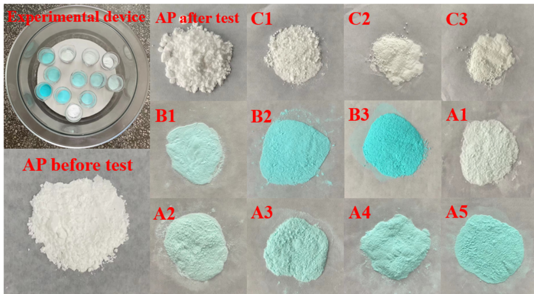
Fig. S10. Diagram of the experimental device and photographs of the individual composite samples after the hygroscopicity test.
