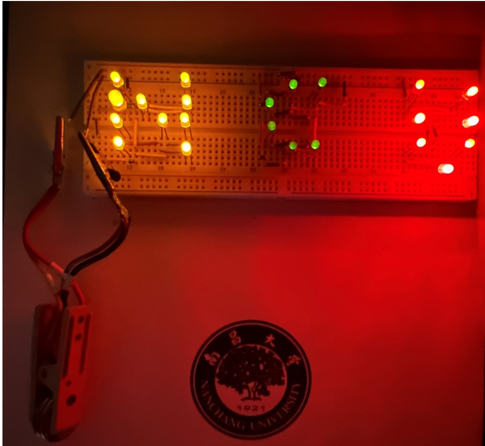
Fig. S15 Photographic image of \text{Ni}_1(\text{Fe}/\text{Co}=1/1)_{0.5}/\text{NF} // \text{AC} HSC device driving LED lamp combination.
