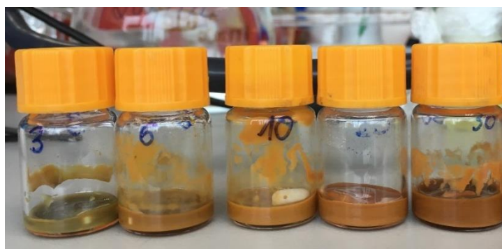
Figure S3. Digital photos taken on the precursor inks containing \text{BiOI} nanoplates powder and \text{VO}(\text{acac})_2 in dimethyl sulfoxide solvent.
