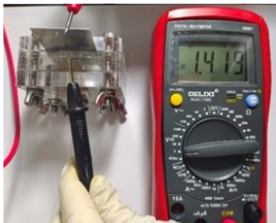
Fig. S9. The homemade zinc-air battery device and the optical photo of open circuit voltage about precious metal 20% Pt+IrO 2 catalyst.
