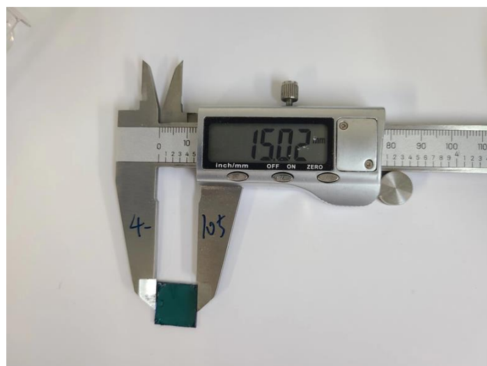
Figure S22. The length measurement of 1.5 cm by 1.5 cm sizes ultra-flexible OPVs (unpeeling off).
