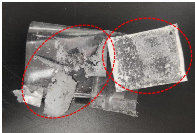
Figure S18. Photograph of the zinc anode from the failed pouch cell after cycling.
