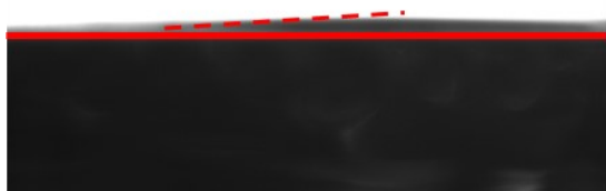
Figure S9. The static contact angle ( \theta < 5^\circ ) between the TiO 2 substrate and the water with PO-2mg
