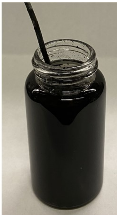
Carbonaceous product detached from cathode by sonication in water
