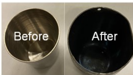
Nickel anode before and after electrospitting
