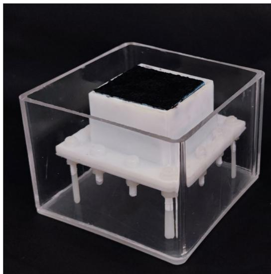
**Fig. S11.** Solar evaporation device with solute replacement.
