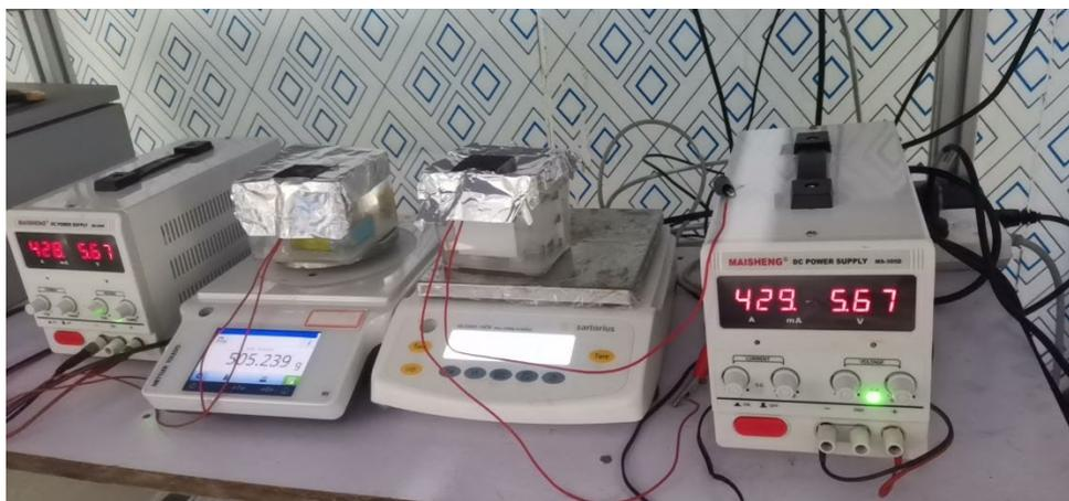
**Fig. S14. Experimental setup for the long-term Joule heating evaporation test.** Two DC power sources were used to provide the same heating power, and the weight of two evaporation systems were measured at the same time. Such test could avoid the difference caused by the unstable ambient temperature and humidity.
