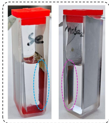
Fig. S18. The side view of the cuvette-type battery cycled.
