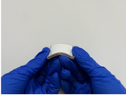
Fig. s8 Photos showing the application potential of the ISRC on curved surfaces. (a) Downward bending. (b) Upward bending. Both PNIPAM hydrogel and SiO 2 fiber have flexibility characters.
