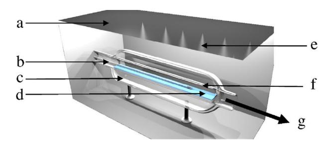
Figure S1. 3D-skatch of (a) stainless steel box, (b) mobile injector, (c) double wall thermostated glass envelope, (d) glass plate covered with the paint, (e) UV lamps (f) the flow tube photoreactor, and (g) exit of the flow gas to the PTR-MS analyzers.
