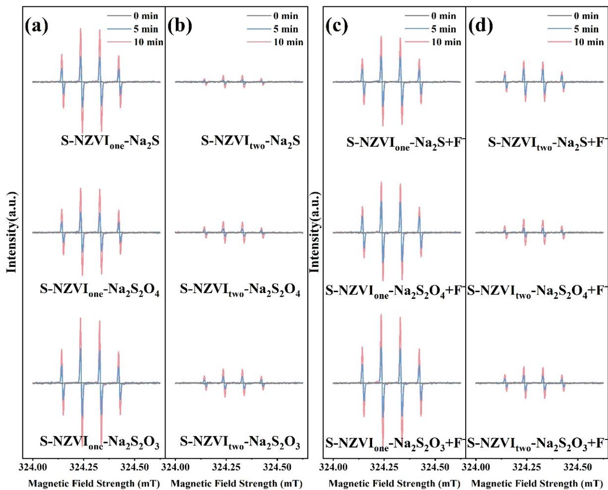
Figure S7. ESR spectra of with DMPO-•OH at 0 min, 5 min, and 10 min for (a) S-NZVI<sub>one</sub> and (b) S-NZVI<sub>two</sub>. ESR spectra of DMPO-•OH at 0 min, 5 min, and 10 min after the addition of 2 mM of F<sup>-</sup> for (c) S-NZVI<sub>one</sub> and (d) S-NZVI<sub>two</sub>.
