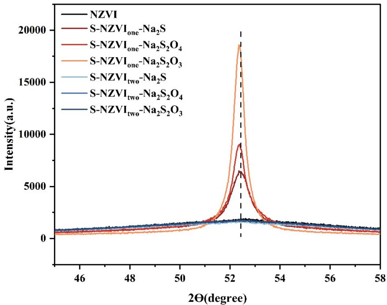
Figure S2. XRD spectra of NZVI and six kinds of S-NZVIs.
