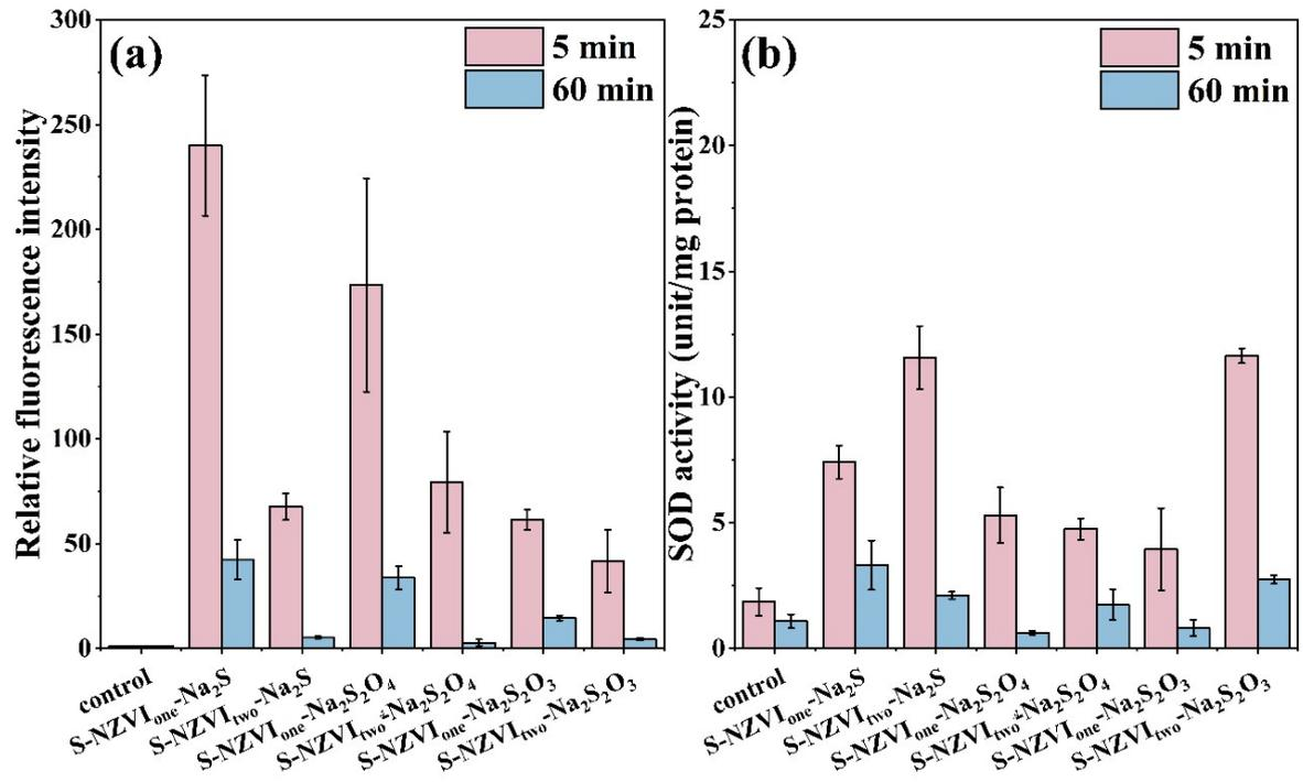
Figure S6. (a) Relative fluorescence values of intracellular ROS at 5min and 60min for six kinds of S-NZVIs. (b) SOD enzyme activity (units/mg protein) at 5min and 60 min for six kinds of S-NZVIs.
