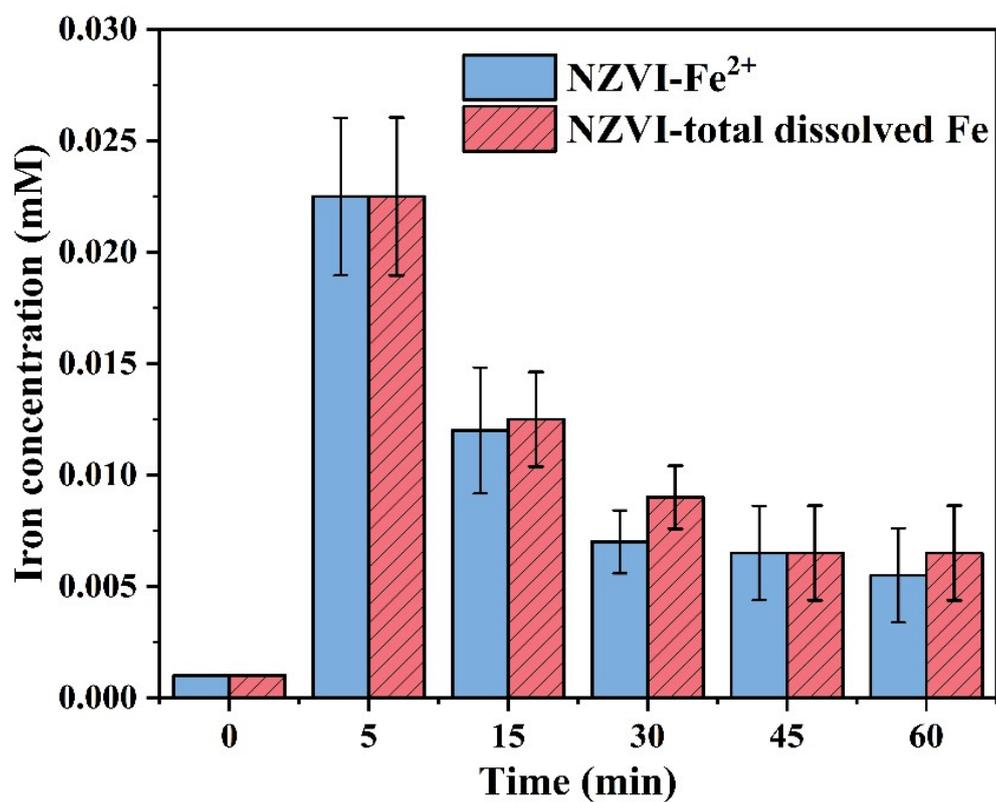
Figure S5. The concentrations of NZVI dissolved Fe<sup>2+</sup> and total dissolved iron at 0, 5, 15, 30, 45, and 60 min.
