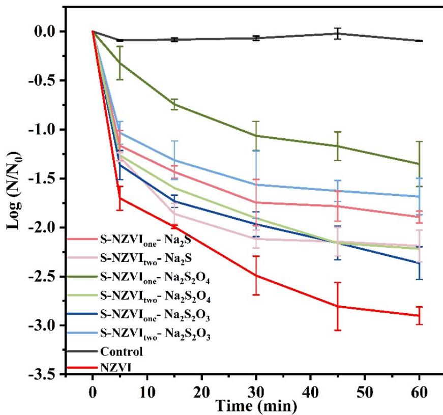
Figure S4. The toxicity of S-NZVI<sub>one</sub>-Na<sub>2</sub>S, S-NZVI<sub>two</sub>-Na<sub>2</sub>S, S-NZVI<sub>one</sub>-Na<sub>2</sub>S<sub>2</sub>O<sub>4</sub>, S-NZVI<sub>two</sub>-Na<sub>2</sub>S<sub>2</sub>O<sub>4</sub>, S-NZVI<sub>one</sub>-Na<sub>2</sub>S<sub>2</sub>O<sub>3</sub>, S-NZVI<sub>two</sub>-Na<sub>2</sub>S<sub>2</sub>O<sub>3</sub>, and NZVI at a concentration of 50 mg/L towards *E. coli* at 0, 5, 15, 30, 45, and 60 min, respectively.
