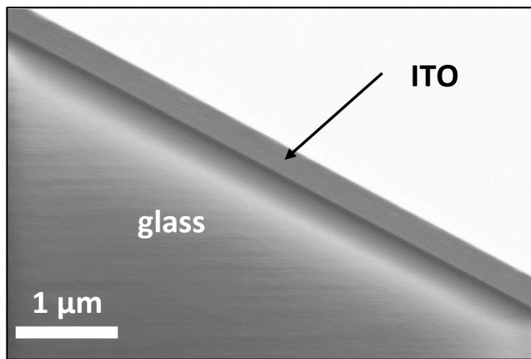
**Figure S1:** Cross-sectional view of the same ITO-coated coverslip obtained by SEM for evaluation of the ITO layer thickness.
