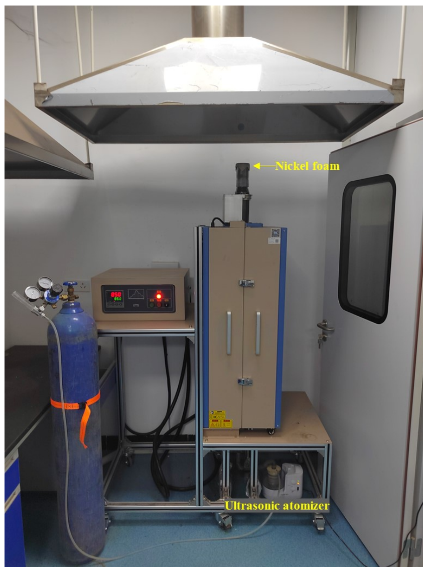
Fig. S2 Photo of the spray pyrolysis device, mainly including a vertical furnace reactor, ultrasonic atomizer, and a powder collector (nickel foam).
