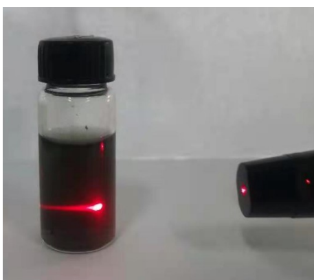
Fig. S4 MXenc 1.0 colloids with the Tyndall effect.
