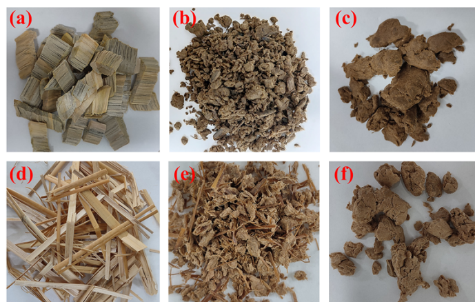
Fig. S1. (a-c) The images of commercial pine chips, coarse pulp, screened pulp. (d-f) The images of reed straw, coarse pulp, screened pulp.
