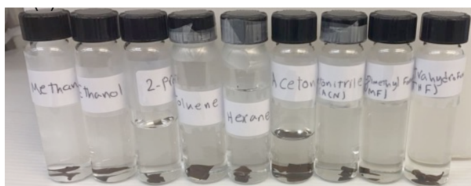
Figure S2. Stability of lignin membranes in ethanol, methanol, isopropanol, acetone, acetonitrile, hexane, toluene, tetrahydrofuran, and N,N -dimethylformamide solution under static condition at 23°C, 8 weeks after soaking.
