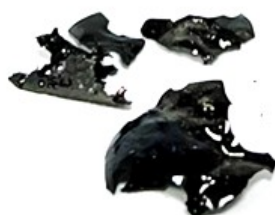
Fig. S6 Digital photos of the polysulfides without addition of BDE (Poly(S-IA)).
