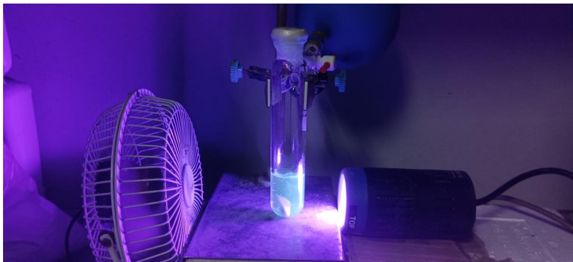
Figure S1. Reaction setups. 0.2 mmol-scale reactor charged with an ethylene balloon (1 atm)
