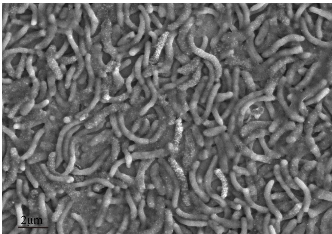
Fig. S2 SEM image of R. rubrum -CdS biohybrid system prepared under a \text{Cd}^{2+} concentration of 0.2 mM.
