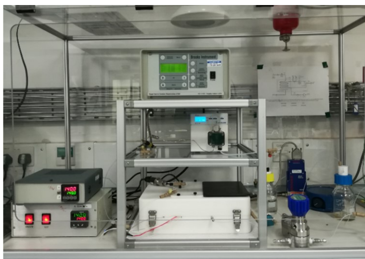
Figure S6. Picture of the slurry loop membrane reactor setup.
