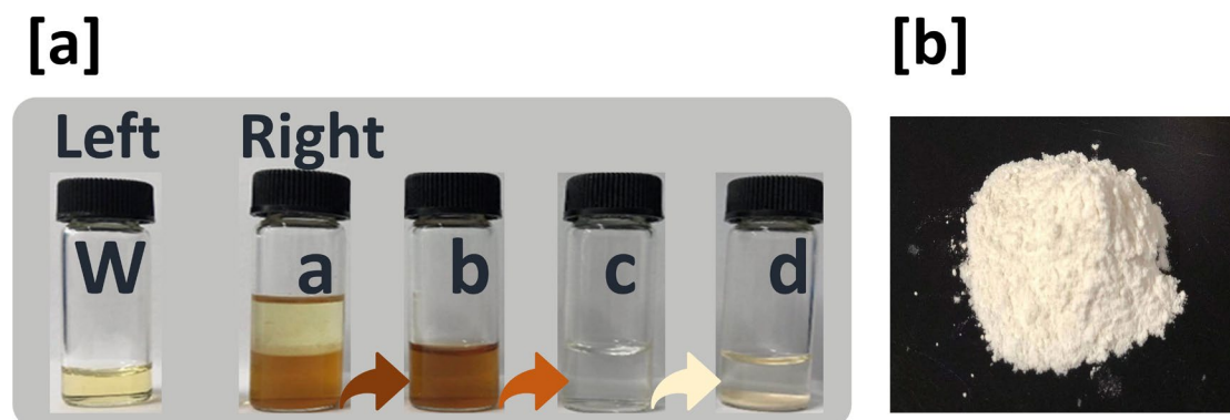
Fig. S10 [a]: Appearance of reaction mixtures during post-processing. Left: W: reaction liquid of aqueous catalytic system after boiling and centrifugal. Right: reaction liquid via a series of post-treatment from the aqueous-organic biphasic catalytic system. a: after boiling and centrifugal; b: aqueous phase though biphasic separation of a; c: decolorized from b by activated carbon; d: CaCl 2 precipitation based on c. [b]: Calcium 5-keto-D-gluconate from bio-oxidation.
