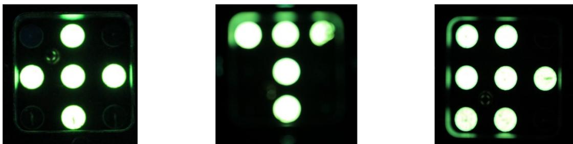
**Figure S20.** The organic light-emitting diode is prepared based on the CSA film.
