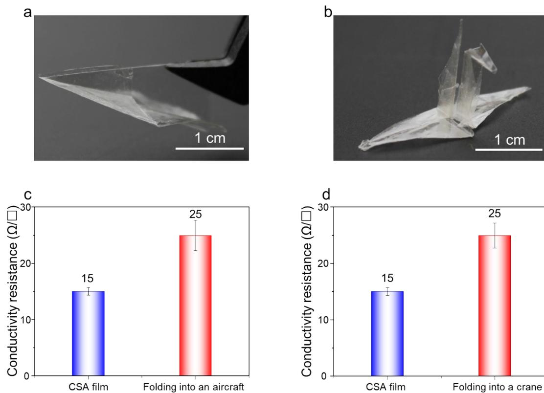
**Figure S11.** The foldability of the CSA film. (a, b) we can fold the CSA film into various shapes, including aircraft shape (a) and crane shape (b). (c, d) The conductive resistance of CSA film with various shapes, including aircraft shape (c) and crane shape (d).
