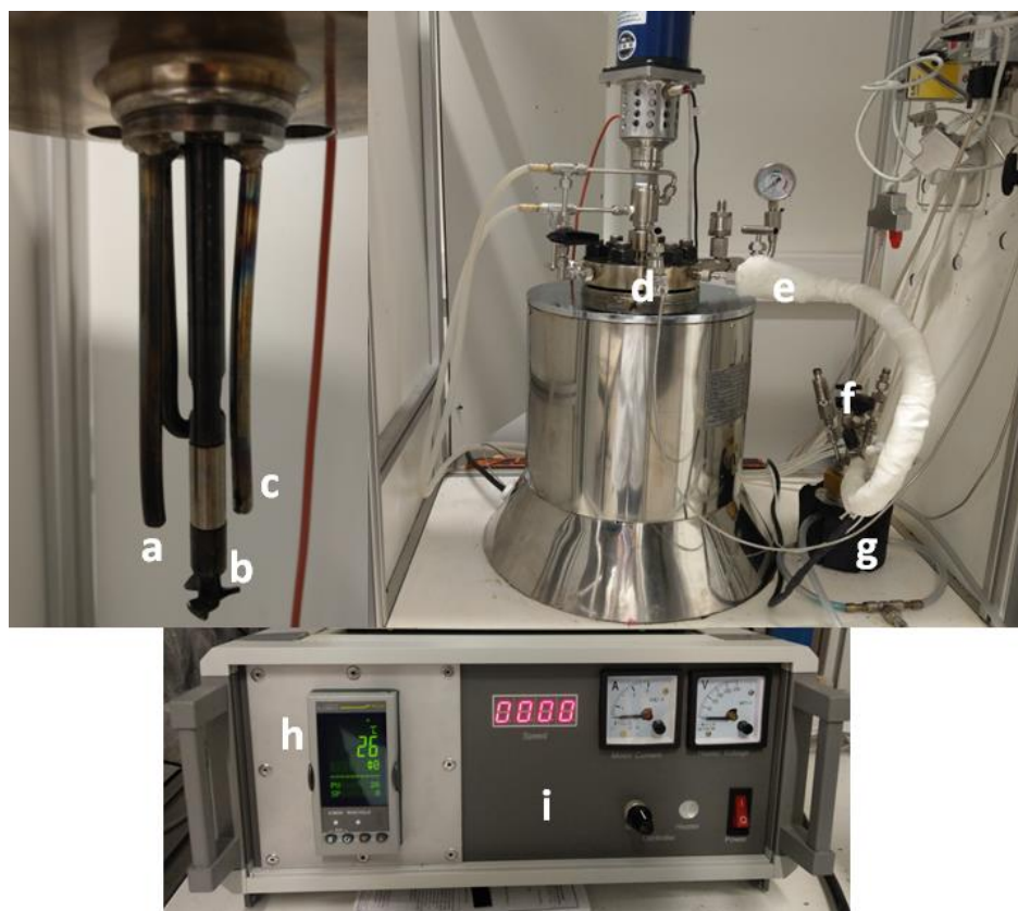
Fig. S1 Pyrolysis reactor: a) nitrogen gas flow dip-tube, b) stirring mechanism c) Pt-100 thermocouple, d) nitrogen flow tube, e) “heated” tube, f) condenser, g) walls of the condenser cooled by an ethylene glycol/water fluid, h) two-loop Eurotherm temperature control system, i) energy supply to the heating elements.
