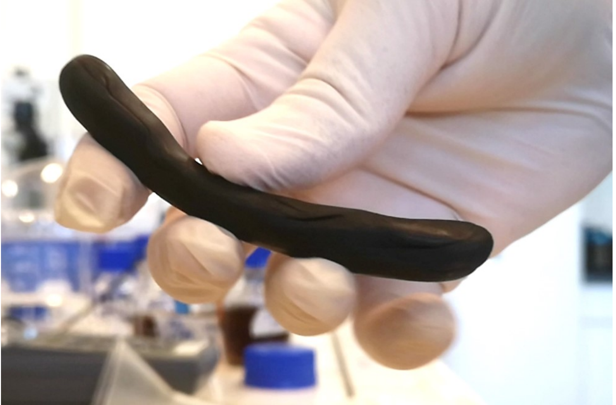
Fig. S6. Extracted suberinic material from cassava peel ( Manihot esculenta ) mild condition.
